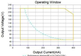
It's important to set the output current (AOC value) according to the LED voltage and make sure the power is within 75 W + 5%.
