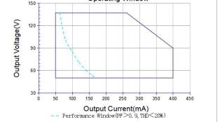
It's important to set the output current (AOC value) according to the LED voltage and make sure the power is within 36 W + 5%.
